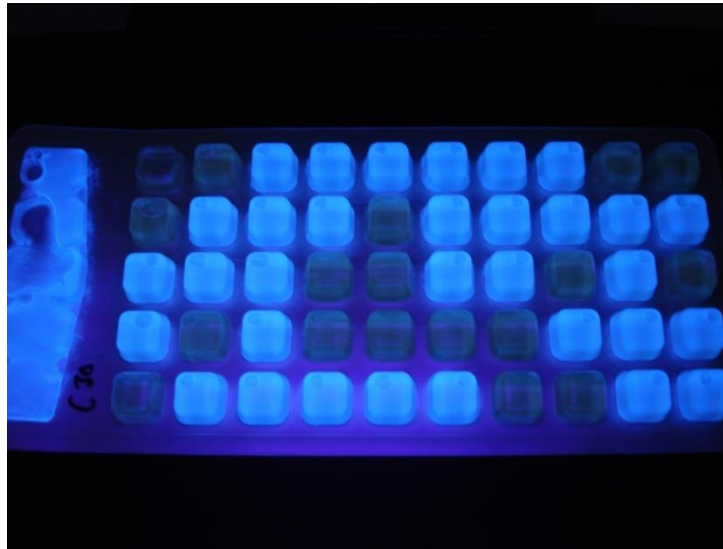
Figure C1 Example of a 51-well MPN reaction pouch (Quanti-Tray®) with a defined nutrient medium (Pseudalert®) with 33 positive fluorescing wells for Pseudomonas aeruginosa
