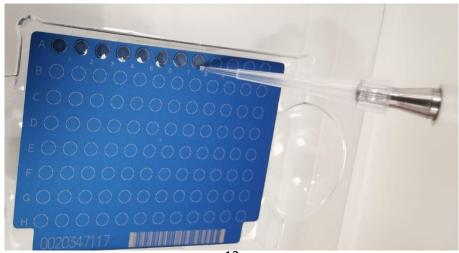
Allow the wells to dry at room temperature. A homogeneous preparation should be observed.
