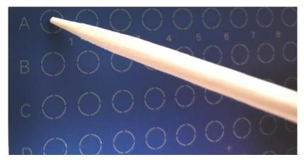
Overlay each of the occupied wells with 1µL of matrix solution. This must be done within the time detailed in the manufacturer's guidance or an appropriately validated time limit.
