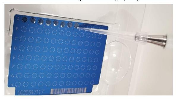
Allow the spots to dry at room temperature. A homogeneous preparation should be observed.
