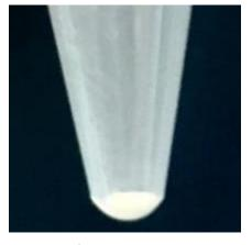
Air-dry the pellet for a minimum of 5 minutes at room temperature.
