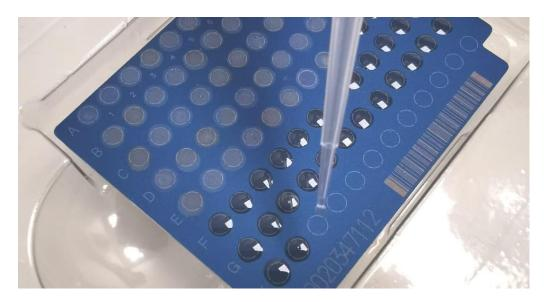
Overlay each occupied well with 1µL of matrix solution. This must be done within the time detailed in the manufacturer's guidance or an appropriately validated time limit.
