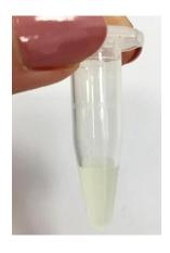
Add 900µl of absolute Ethanol to the microcentrifuge and mix thoroughly using a vortex.
