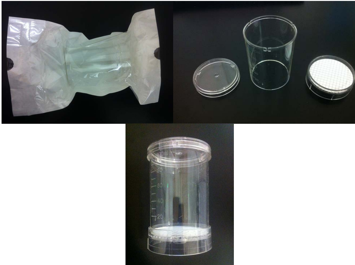
Figure 6.9.2 Disposable plastic filter units
