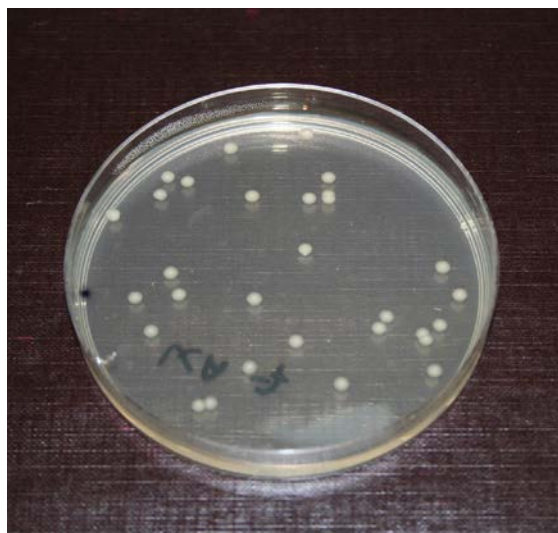
Figure 6.10.4 Quantitative quality control – E. coli growing on nutrient agar giving a direct count
