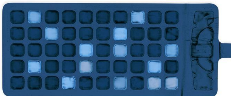
Figure E2 Example of MPN reaction pouch with a defined substrate medium with 14 fluorescing wells showing presence of E. coli
