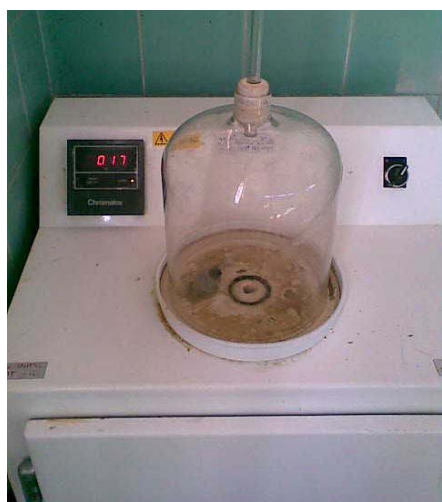
Figure A4.1 Typical apparatus for the assessment of odour - smell-bell
