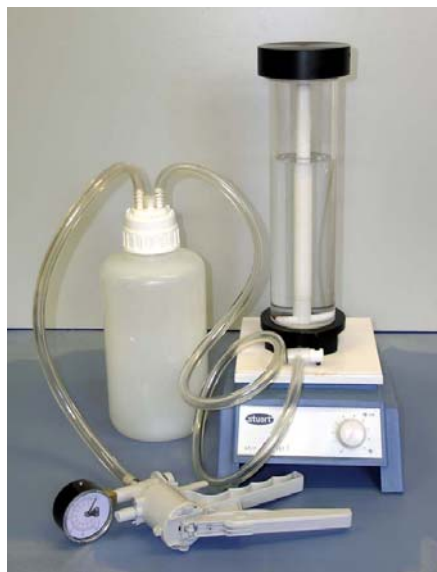
Figure A8 Filta-Max® concentration tube set with stirrer assembly, on a magnetic stirrer and connected to a catch-bottle and vacuum pump
