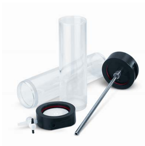
Figure A7 Elution tube (standing - threaded at one end) elution base (with stainless steel tube attached) concentrator tube (laying - threaded at both ends) and concentrator base (with tap)
