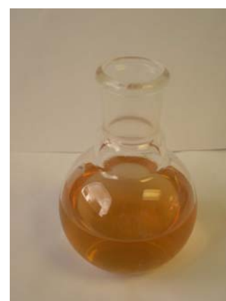
Immediately following titration end-point
