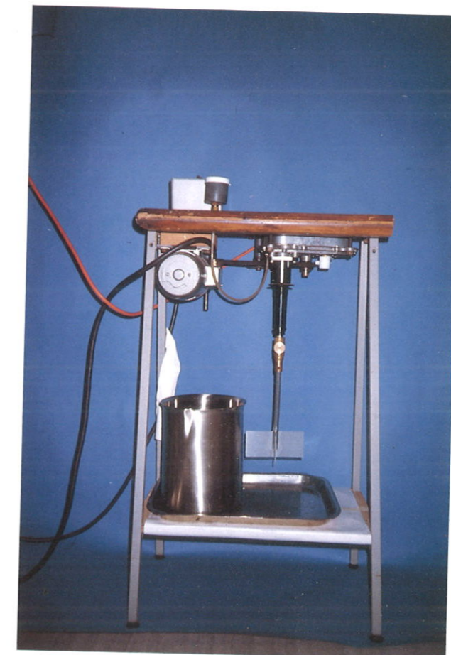
Fig. 19. Stobhill Washing Machine. Container removed to show the ultrasonic vibrator.
