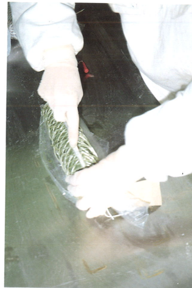
Fig. 2a. Cutting open a Cuno filter for Cryptosporidium and Giardia.
