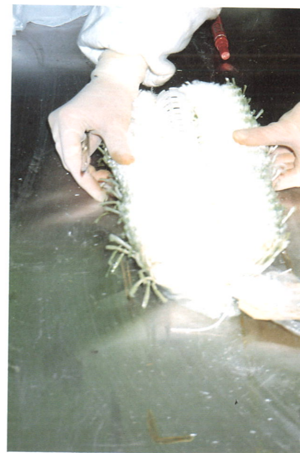
Fig. 2b. Teasing open a Cuno filter for Cryptosporidium and Giardia.
