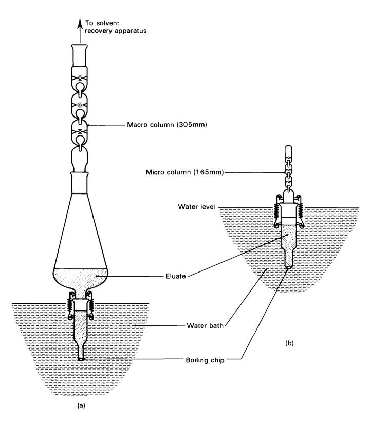
Figure 3 Sample clean-up apparatus
