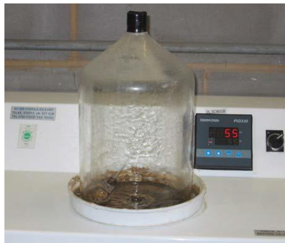
Figure A4.1 Typical apparatus for the assessment of odour - smell-bell
