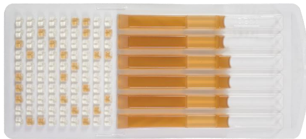
Figure C1 Example of a 96-well MPN Quanti-Tray®/Legiolert™ 96-well reaction pouch with Legiolert™ with the 6 large wells and 24 small wells showing brown colouration for Legionella pneumophila
