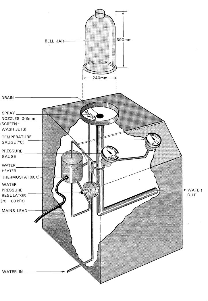
Fig. 1 Cutaway view of an apparatus for the assessment of Odour - Smell Bell
