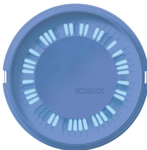
Figure 1 Example of a 50-well reaction module for the enumeration of heterotrophic plate count bacteria with 35 wells showing blue-white fluorescence
