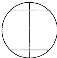
(ii) Systematic pattern used to scan the whole base of a sedimentation chamber
