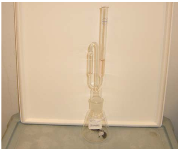
Figure E1 Glass bubbling equipment for collecting evolved gases
