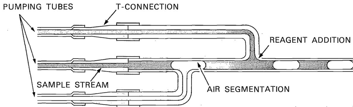
FIG 19 T-CONNECTIONS REAGENT ADDITION AND MIXING
