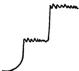
Observed when initially calibrating the detector with a standard solution; caused by a dry membrane and ageing membrane
