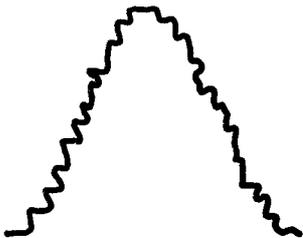
Insufficient gain (amplification) on the recorder
