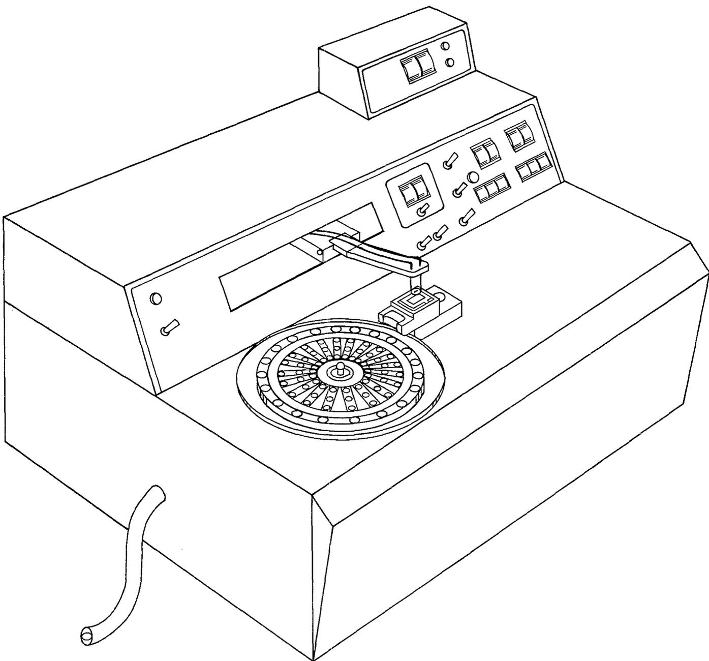
Figure 2 Schematic representation of a centrifugal analyzer rotor
