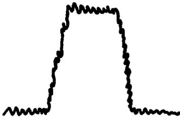
Poor quality reagents or air bar out of sequence
