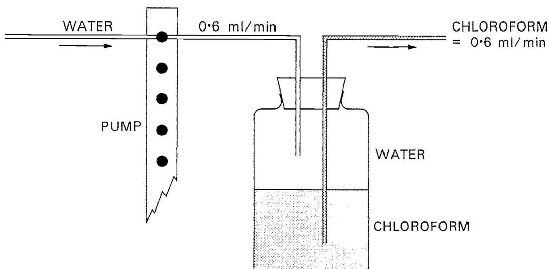
FIG 16 ALTERNATIVE DESIGN OF THE PERISTALTIC PUMP
