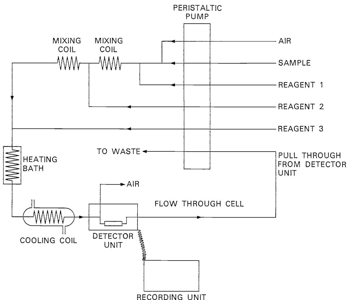
FIG 10 LINE (FLOW) DIAGRAM OF AN AIR-SEGMENTED CONTINUOUS FLOW AUTOMATIC ANALYSER
