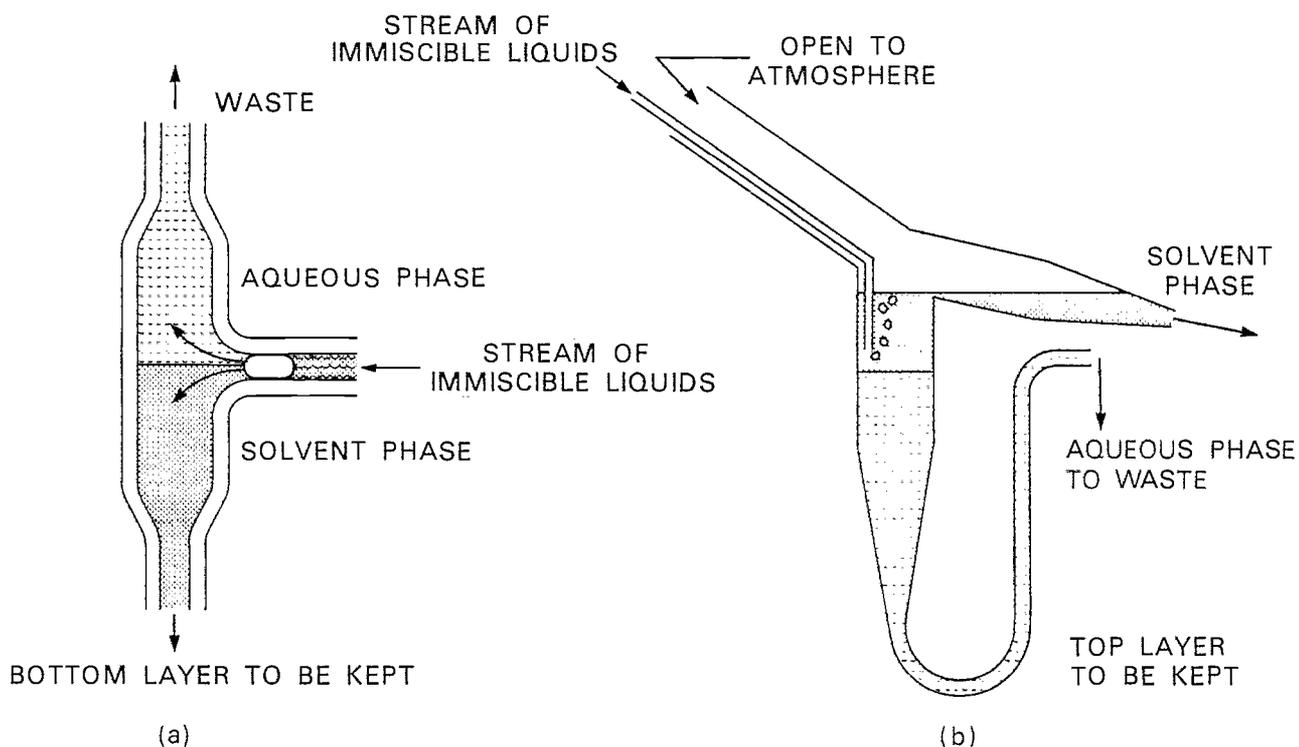
Figure 21 shows a typical debubbler for a colorimetric measurement. Other measuring devices which require a bubble free sample may be inserted into the detector cell. The detector cell volume should be small enough to contain less than the solution resulting from one sample at any one time, regardless of detector type used.
