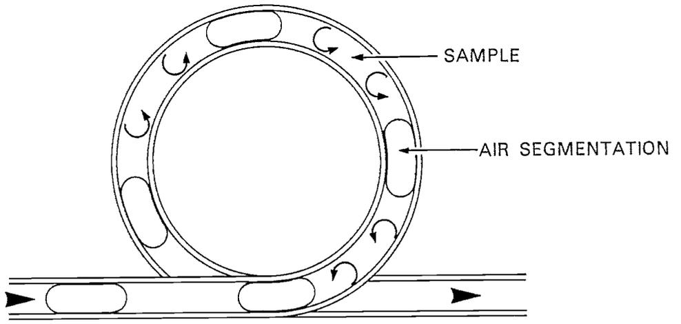
FIG 17a FUNCTION OF A TYPICAL MIXING COIL
