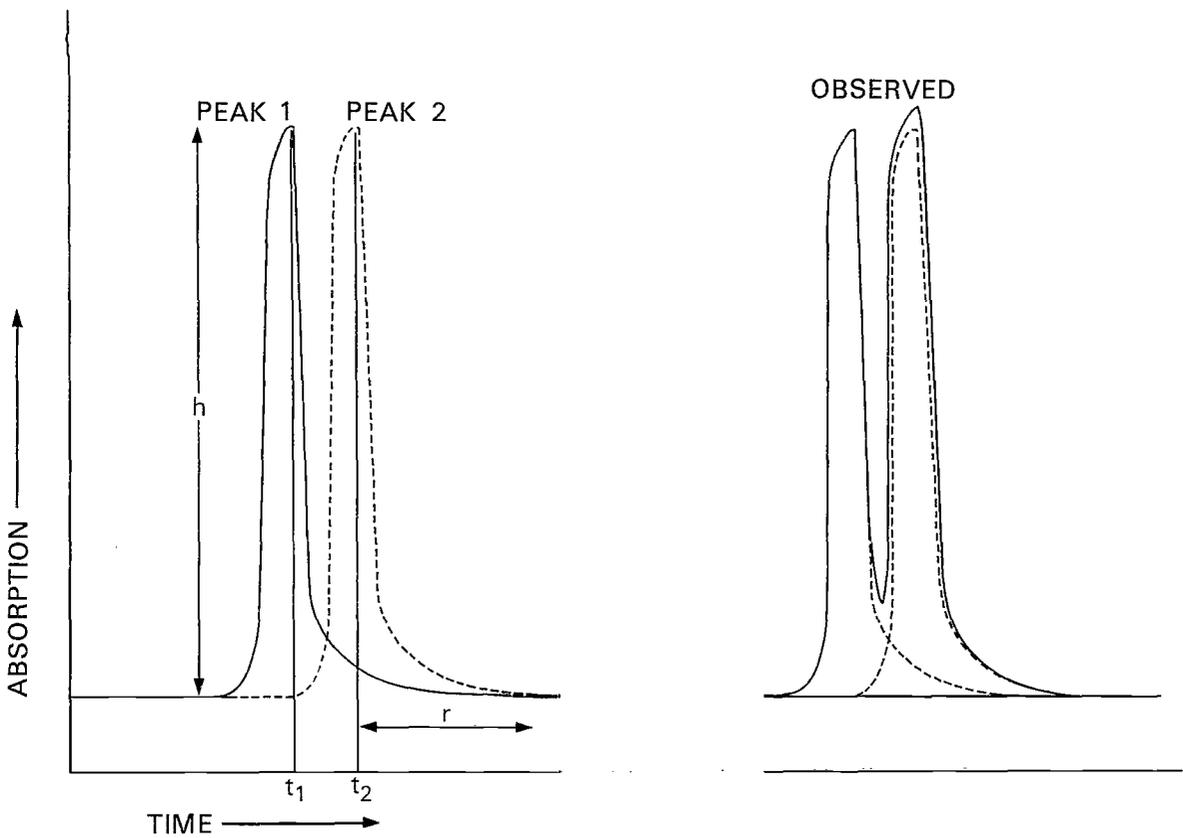
FIG 24 A TYPICAL ABSORPTION CURVE ILLUSTRATING THE EFFECT CARRY OVER WILL HAVE ON A SUBSEQUENT CURVE (SEE ALSO FIG 23)
