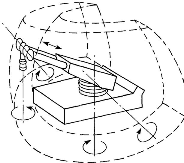
The arm slides in and out as well as rocking up and down and to and fro. The head may itself also rotate.
