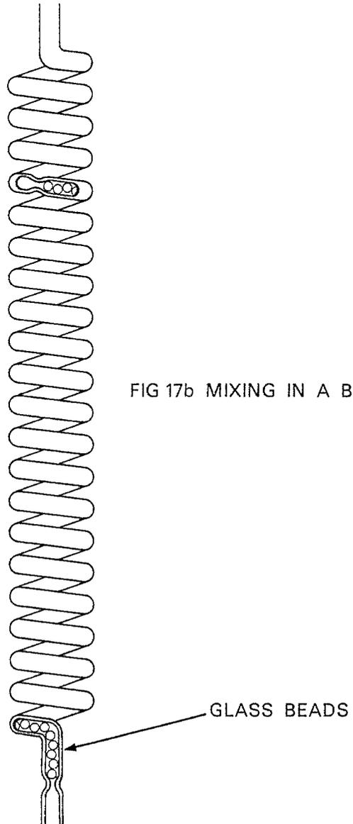
FIG 17b MIXING IN A BEADED COIL
