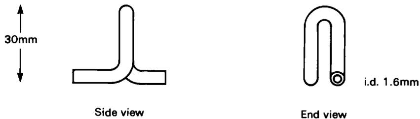
Figure D3 Detail of plating trap (alternative)
